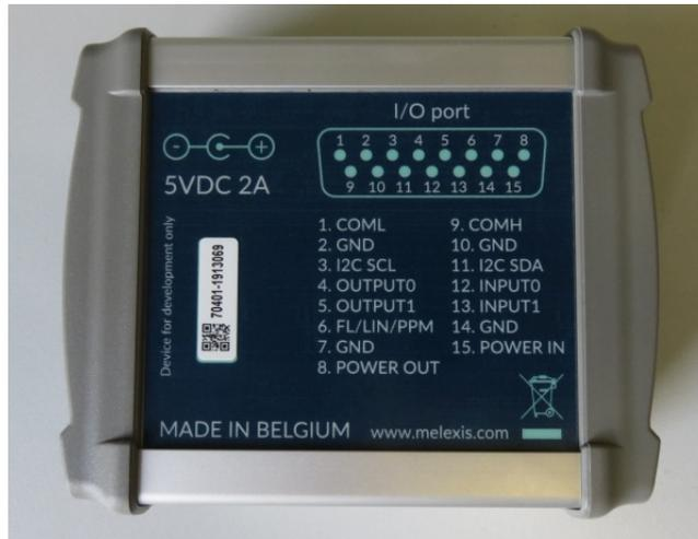
Figure 11: Pin configuration of the D-SUB15 connector
